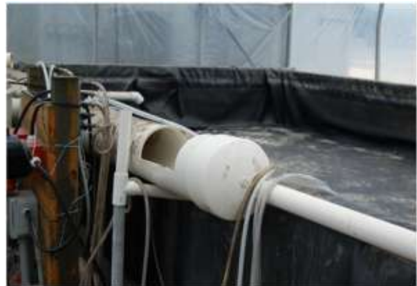
30 m 3 nursery tank in greenhouse immediately adjacent to the greenhouse housing the growout raceway, and the chute by which juveniles are transferred to the raceway.
