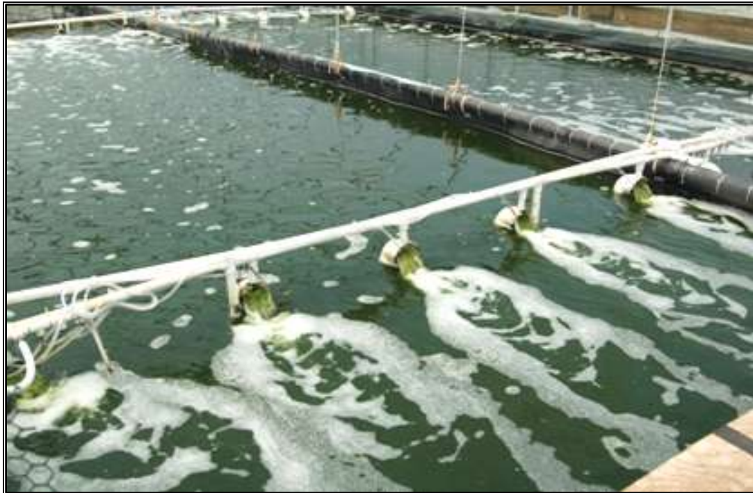
56 airlifts mix and circulate the water, preventing solids from accumulating on the bottom, providing aeration, and distributing injected oxygen throughout the system.
